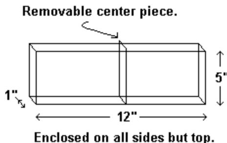
\* A workable device has been constructed with from a plastic shoe box with a center piece cut from a milk carton held in place by toy modeling clay although a thinner trough seems to work a bit better. A commercial version of this device is available from Flynn Scientific Inc., P.O.Box 219, Batavia, IL, 60510 catalog #AP4784 for about \$30.00
