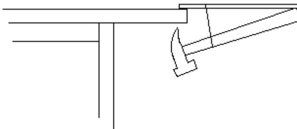
This works because the center of mass (somewhere near the hammerhead) is under the supporting end of the ruler on the tabletop. It looks impressive because the majority of the ruler and handle is suspended off the edge of the table.
